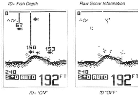
"ID+", the default setting, provides more information about the location of the target by attaching depth "strings" showing the digital depth of the target. When there are numerous targets on-screen, not every target depth is shown, to avoid excessive clutter on-screen.
