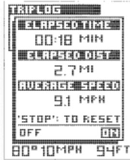
Note: The optional Temp/ Speed accessory must be connected for Triplog to work.
