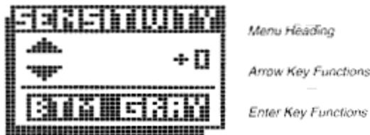
All menus use the same general layout as shown in the sample men at the right. The heading of the menu is at the top. The area in the center is controlled by the UP and DOWN arrows, and the area under the horizontal line is controlled by the ENTER button. Not all menus are affected by all controls, but the layout is the same regardless. Pressing MENU repeatedly will sequentially display all available menus.
