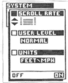
User Level is used to select Normal or Advanced operation. Advanced Mode performs several functions which will benefit the experienced user. Icons are not shown and numerical data is smaller to allow more of the display to be used for the picture of the bottom. Several other changes in operation occur which are designed to increase the speed of adjustments, and maximize the graphic use of the display.
