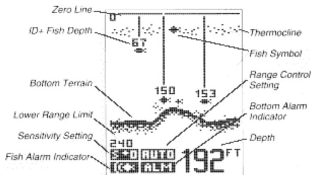
There are three basic screen layouts for the Wide W. Figure A shows the default screen layout which does not include temperature and speed readings. If you have purchased the temperature and speed accessory and it is installed, the screen layout will be slightly different as shown in Figure B.
