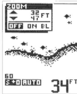
To enable Zoom, adjust the depth of the zoom range first using the UP and DOWN arrow buttons until the upper and lower limit numbers correspond with the range you wish to view, then enable Zoom using the ENTER button.
