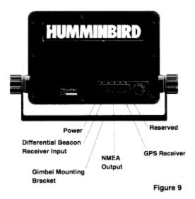
Gimbal Mounting Bracket: Allows the NS 10 to be adjusted to the optimum viewing angle. To adjust, loosen the knobs on the gimbal mounting bracket and adjust the unit for best visibility. After adjusting, tighten the knobs and the unit will stay in position.
