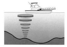
The LCR 400ID uses the returned signals to display a detailed underwater image, and constantly updates the display as you travel across the water. The display informs you of the current depth and reveals individual fish, schools of fish, their location, and bottom details.
