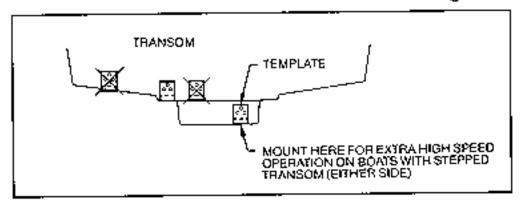
NOTE: On boats with more than 15 degree deadrise angle it may be necessary to mount the transducer slightly off parallel with the water level. (See Figure E)
