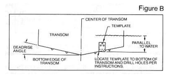
Once the location is determined mark and drill three 7/64" dia.. holes noted on the template. Attach the metal bracket using three #10 self threading screws supplied. Be sure to align holes in the center of the
