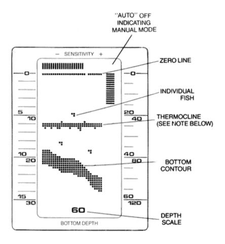
Thermocline is a temperature change at a certain depth in the water. In some conditions the sonar waves will actually reflect or bounce off this temperature change and therefore it will be displayed on the LCR as shown above. To see the thermocline, you will need to go to the manual mode and increase the sensitivity setting.
