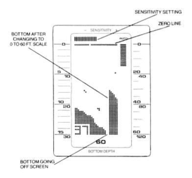
TROUBLE SHOOTING: If the display comes on when the "On" button is pushed but no bottom information is seen, check that the transducer connector is securely locked to the rear of the LCR. Also insure that the transducer is completely submerged. A transducer cannot work properly in air or through air bubbles in the water.
