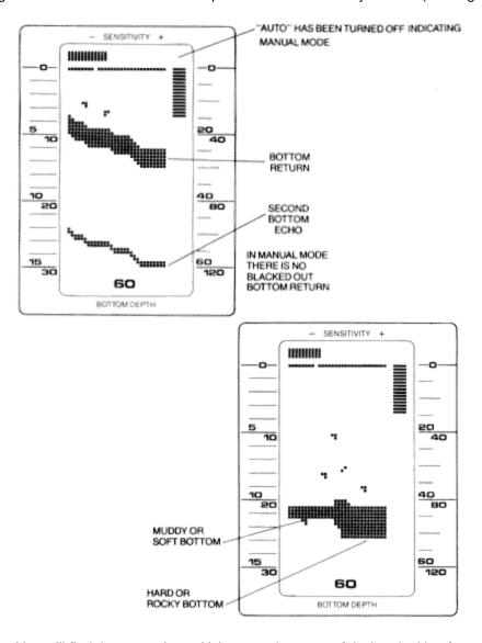
Note: You will find the manual sensitivity control most useful when looking for smaller targets such as smaller fish. In the automatic mode the computer might not be using enough sensitivity to show smaller targets. At higher sensitivity settings more targets will be seen. Therefore, you might want to use the automatic mode while running and then use the manual mode for charting and finding fish.
