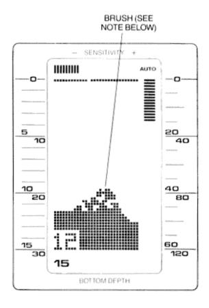
Brush or thick standing timber will appear as a thick mass with holes or gaps as shown above.
