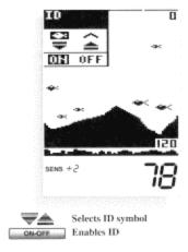
ID identifies targets not attached to the bottom and displays them with either a fish symbol or an arch. Three different size symbols are used to represent the returned signal strength, a good indicator of fish size. Use the up and down arrow keys to switch between fish or arches, or use the ON-OFF key to disable ID.
