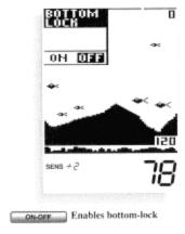
Bottom-Lock provides an up-close view like Zoom Range, except that in this case the zoomed view automatically moves up or down to stay on the bottom. To use this feature, select BOTTOM LOCK and press ON-OFF. The range of the display is shown when Bottom-Lock is on.
