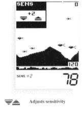
The LCR 120 automatically adjusts to the proper amount of sensitivity for conditions (i.e. depth). You can bias the setting + or -5 levels to suit your personal taste. Increasing the sensitivity targets and the thermoclines, which might not be displayed at the +0 setting. If you want to manually adjust Sensitivity, select SENS and press the Up or Down arrow button to adjust the display.
