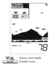
Zoom Range provides an up-close view. To activate it, select ZOOM RANGE and press ON-OFF. The Zoom view begins initially at the surface; press the Up or Down arrow to adjust Zoom Depth. The range of the display is shown when Zoom is on.
