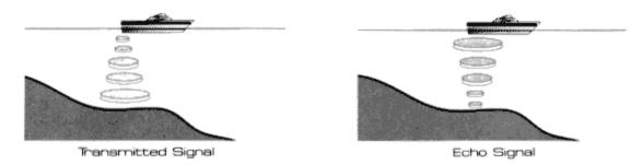
The transducer and LCR 100 use the basic principles of sonar to reveal objects beneath the water's surface. The LCR 100 continuously sends electronic signals to the transducer, which converts them to ultrasonic signals that it aims toward the bottom. Each signal travels downward until it strikes an object or the bottom, then immediately echoes back to the transducer. As the transducer receives these signals, it converts them back to electronic signals for display on the LCR 100 screen.
