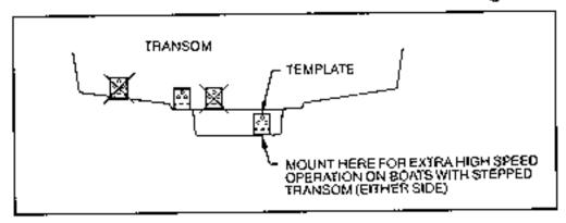
NOTE: On boats with more than 15 degree deadrise angle it may be necessary to mount the transducer slightly off parallel with the water level. (See Figure E)
