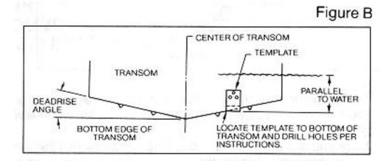
Once the location is determined mark and drill three 7/64" dia.. holes noted on the template. Attach the metal bracket using three #10 self threading screws supplied. Be sure to align holes in the center of the
