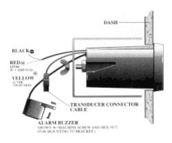
ignition is turned on. No fuse is necessary on the yellow lead. If your boat does not have a switchable electrical system, you must wire the yellow lead through a separate switch, then directly to the power source.
