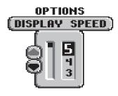
Use the UP and DOWN ARROWS to select the desired update rate. (1) is the slowest, (5) is the fastest. Use the MENU button to advance to the next menu.
