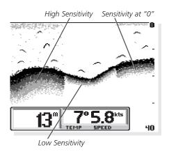
In murky or muddy water, it is often helpful to reduce the sensitivity. This prevents the display from being cluttered with sonar returns from debris or suspended particles. In very clear or very deep water, it may be helpful to increase the sensitivity since even the smallest sonar return may be of interest to the user.
