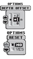
**Reset.** With the many User Options available to customize the *4255X*, it is easy to configure the unit in such a way that it is detrimental to a particular use. By using the Reset function, all variable or user-controlled features of the *4255X* are returned to the factory settings.
