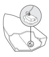
Inside the Hull Mounted Transducer
