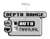
Arrow Keys. The UP ARROW and DOWN ARROW make adjustments to menu functions. On the left side of every menu there are UP ARROW and DOWN ARROW symbols. The symbols indicate which ARROW button has a function in a particular situation. Either one or both ARROW buttons can be used to adjust the menu function. A hollow ARROW symbol means the
