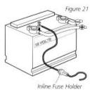
The Power can be connected to the boat's electrical system at two places: a fuse panel, usually located near the console, or directly to the battery.
