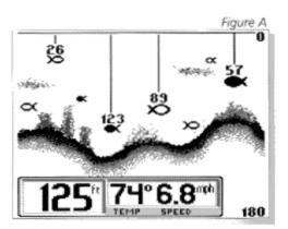
Temperature/Speed. The initial screen layout takes one of two basic forms depending on whether the optional Temp/Speed accessory is installed. Figure A shows the default view when the Temp/Speed accessory is installed. Figure B shows the default view when the Temp/Speed accessory is not installed.
