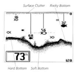
depiction is narrow and dense. If the bottom is soft mud or sand, the depiction will be thick and less dense. This indicates that much of the signal is absorbed by the soft bottom. If the bottom is rocky or rugged in composition, the depiction is of varying density and textured in appearance.
