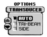
If a faulty transducer is connected, the 400TX may not change the screen presentation to match the transducer. In this instance, you may need to manually select
