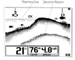
the driver seat facing forward). Hollow fish symbols facing to the left are detected in the left beam, and thus the fish is to the left side of the boat. Solid fish symbols represent fish in the single center beam, and these fish are directly under the boat
