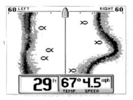
View button. The default view is both, in which information from both the left and right elements are displayed on screen. The digital depth of the water beneath your boat is always present.
