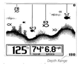
Using manual Depth Range control, you can view sonar information from the area near the surface in great detail.
