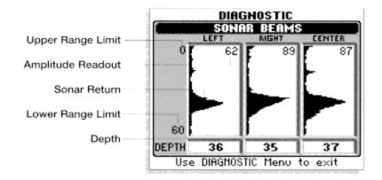
By referring to this screen prior to permanently mounting a through-the-hull transducer, the location can be adjusted until no visible loss is observed.
