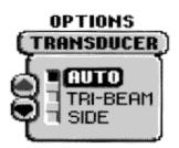
Transducer. The Transducer Option controls the 400TXs ability to determine the transducer connected. If you are using the standard tri-beam transducer or wide side transducer, no adjustment to this menu is needed unless the transducer develops a fault, which is a rare occurrence. The factory setting for the Transducer menu is "Auto". The transducer menu selections will be remembered when the 400TX is turned off.
