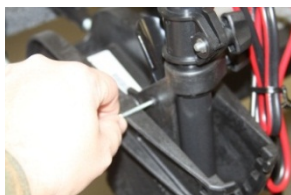
Figure 18: Tilt Lever Pin being pushed into position
