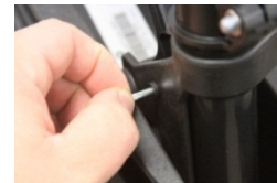
Figure 5: Knurls exposed removing Tilt Lever Pin by hand
