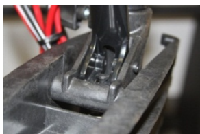
Figure 17: Tilt lever in place without Tilt Lever Pin
