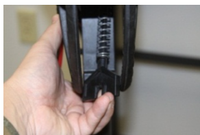
Figure 12: T-bar being guided out of bracket assembly
