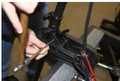
Figure 3: Start of removing the Tilt Lever pin
