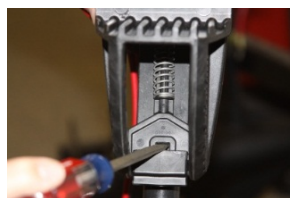
Figure 7: Pry bar positioned to lift T-Bar
