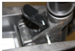
Figure 19: Tilt Lever Pin ready to be driven into place
