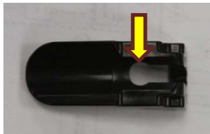
Figure 10: Close up of Tilt Lever, wider portion of opening indicated by arrow
