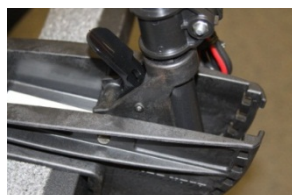
Figure 20: Tilt Lever Pin fully installed
